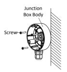
Figure 2-5 Fix the Camera to the Ceiling
