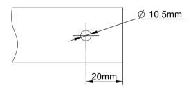
When drilling new holes always ensure they are diametrically opposite each other so that the bolt can pass straight through.
