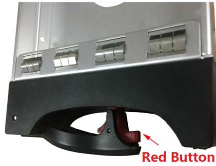
Figure 2-10 Open the handle
