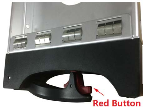
Figure 2-1 Opening the handle
