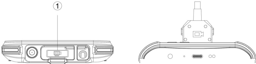
For helmet camera, install the camera at the right side of the helmet.
