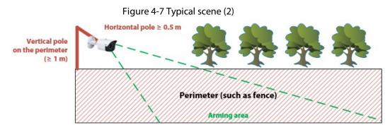
• When there are obstructions (such as trees and vegetation) around the perimeter, and wire netting on the perimeter, install a vertical pole separately. Keep the pole 1 m from the perimeter, and 1 m higher than the perimeter (installation height 3 m-5 m).
