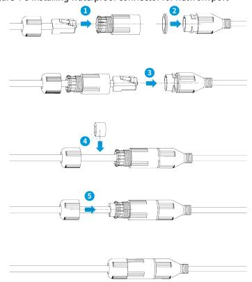
Figure 4-3 Installing waterproof connector for network port
