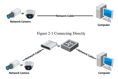
Figure 2-2 Connecting via a Switch or a Router
