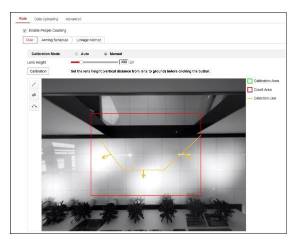
Figure 4-2 Manual Calibration
