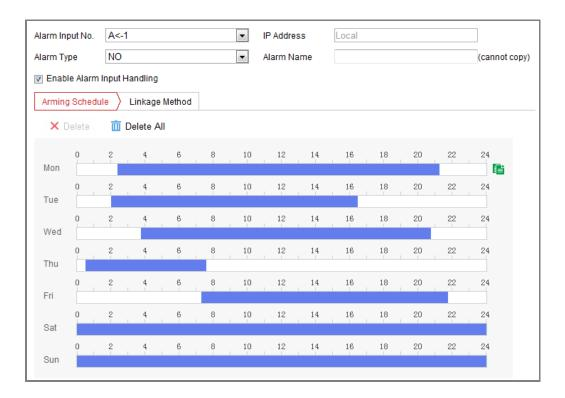
Figure 10-2 Alarm Input Settings
