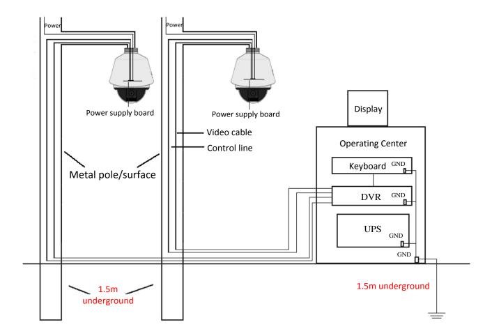
Figure A.3.4 Grounding in Metal Pole Installation
