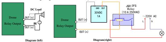
Figure A.9.1 Alarm Out Connections
