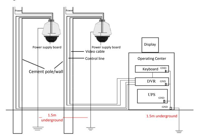
Figure A.3.3 Lightening-protection Grounding in Cement Pole/Wall Installation
