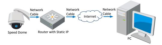
Figure 2-10 Accessing the Speed Dome through Router with Static IP
