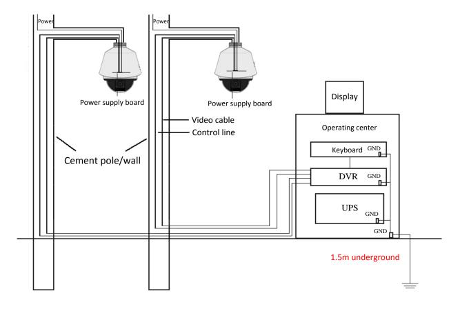
Figure A.3.2 Grounding in Cement Pole/Wall Installation
