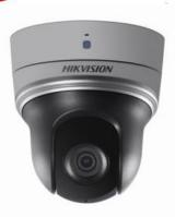
This IR Mini PTZ Camera shows the easy installation, adjustment, and maintenance. It is a camera for indoor area such as the café, hotel, office lobby, small shop, etc. In addition, DS-2DE2204IW supports 4x zoom, Hik-Connect, and PoE & 12VDC power supply. Embedded with 1/2.8" progressive scan CMOS chip makes DWDR and 2.0MP real-time resolution possible. With the pan/tilt, 4x zoom Day/Night IR cut filter, and the IR lights, the camera offers more details in the indoor environments.
