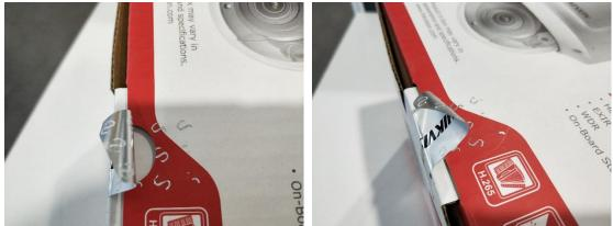
Figure 2 Tamper seal sample after a tampering attempt
